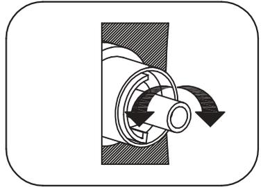
Turn the spindle until the 38 °C is achieved, once this has been reached ,replace the handle, so that the stop pin inside sits against the stop ring.
