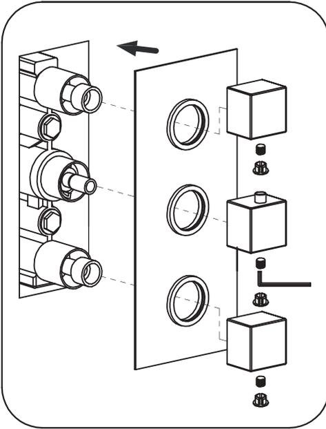
Once the mixer has been fitted and secured, push the concealing plate over the mixer body, sealant should be applied between the plate and the wall.
