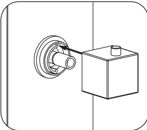
Fit temperature control handle to thermostat, ensuring the stop pin inside the handle, is located against the top of the stop ring.
